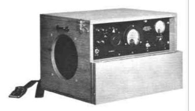
The Type 559-A Noise Meter of 1933 opened up a new field of measurement, acoustics, in which the company has remained preeminent.
